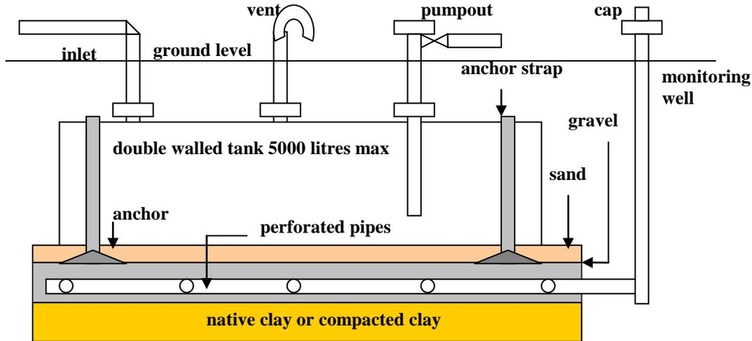
**Underground Storage Tank System Leak Detection System Top View**
