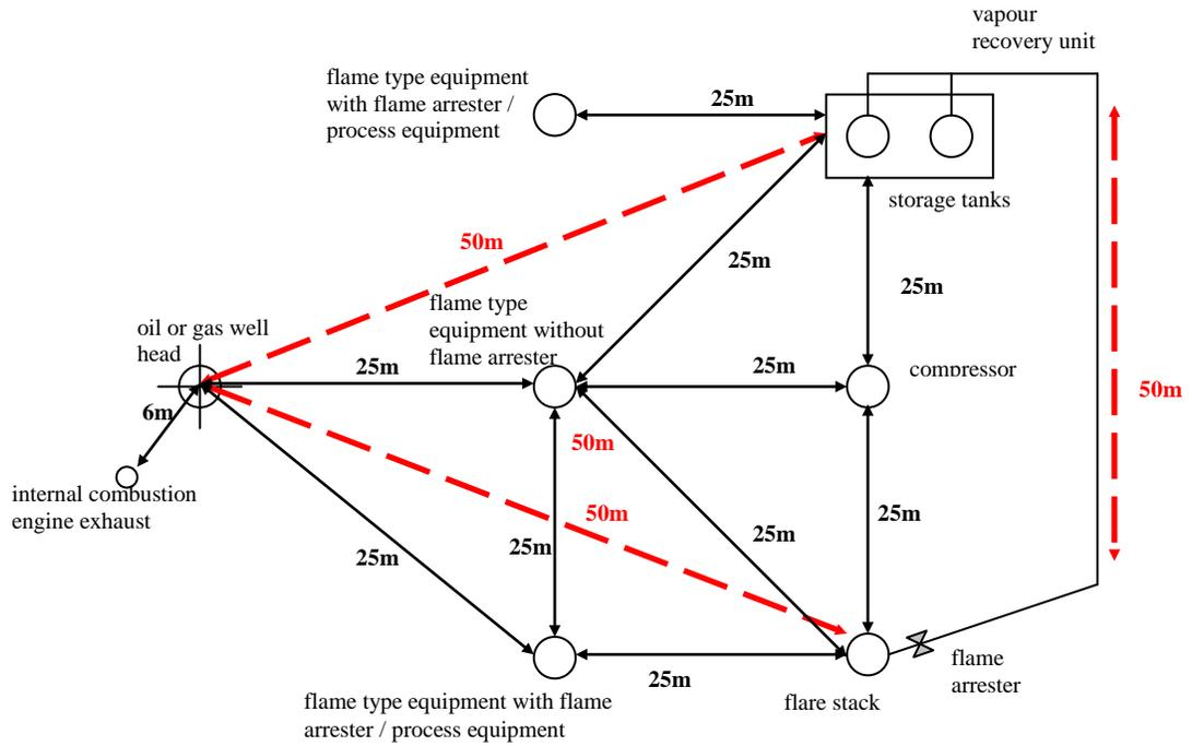
Dashed (Red) Line = 50 metres, Solid (Black) Line = equal to or greater than 25 metres, No smoking within 25 metres of well head, separator, oil storage tank or unprotected source of ignitable vapour
